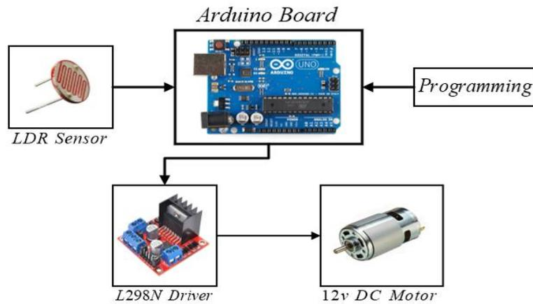
Fig 1: Block diagram of Solar Tracker System
