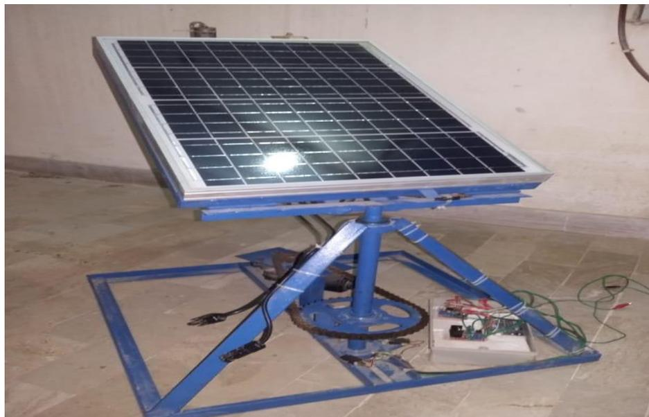
Fig 2: Hardware Model of Solar Tracker
