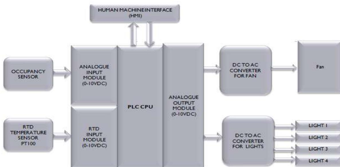
Fig1. BLOCK DIAGRAM OF SMART PLC SYSTEM
